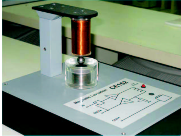
Figure 5.1: Model of the magnetic levitation system.
